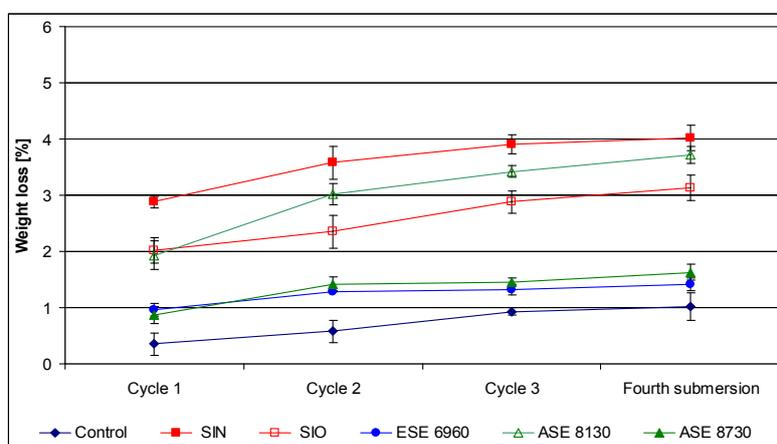
**Figure 6. Weight losses after the water submersion and cyclic tests of silicone treated veneers**
