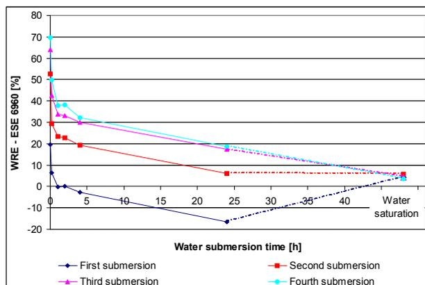
**Figure 5. Water repellent effectiveness of epoxy functional polysiloxane ESE 6960 treated veneers**
