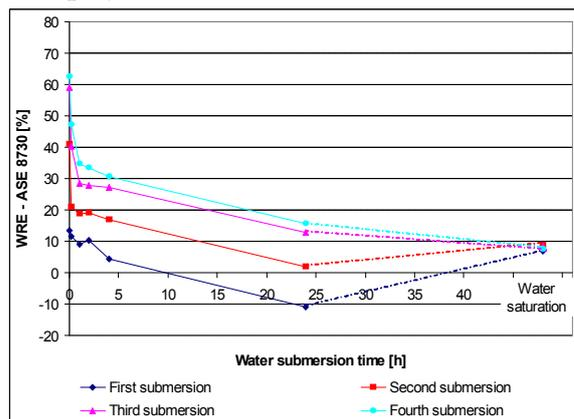
Figure 4. Water repellent effectiveness of amino functional polysiloxane: ASE 8130 and ASE 8730 treated veneers
