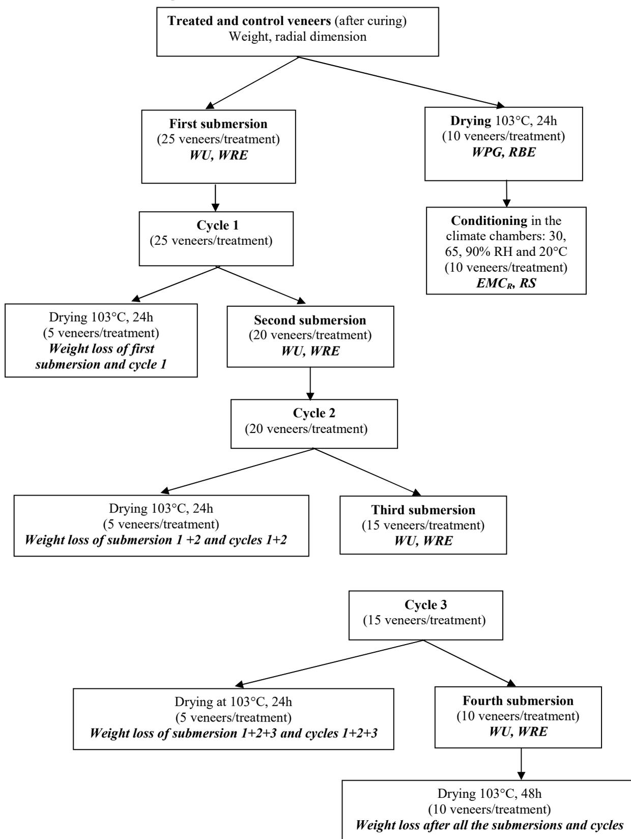
Figure 2. Test procedure of the treated veneers
