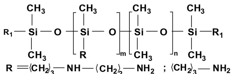
**Figure 1. Chemical structure of polysiloxane with amino groups**
